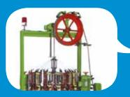
• Fully electronically controlled take up mechanism, with the take off discs up to 1200 mm
